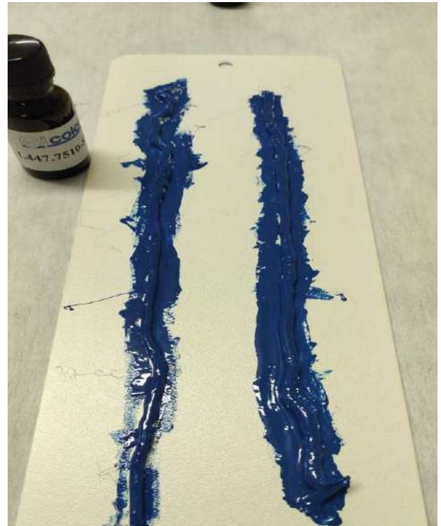
Figure 12-13: Touch-up paint application on silicone sample
