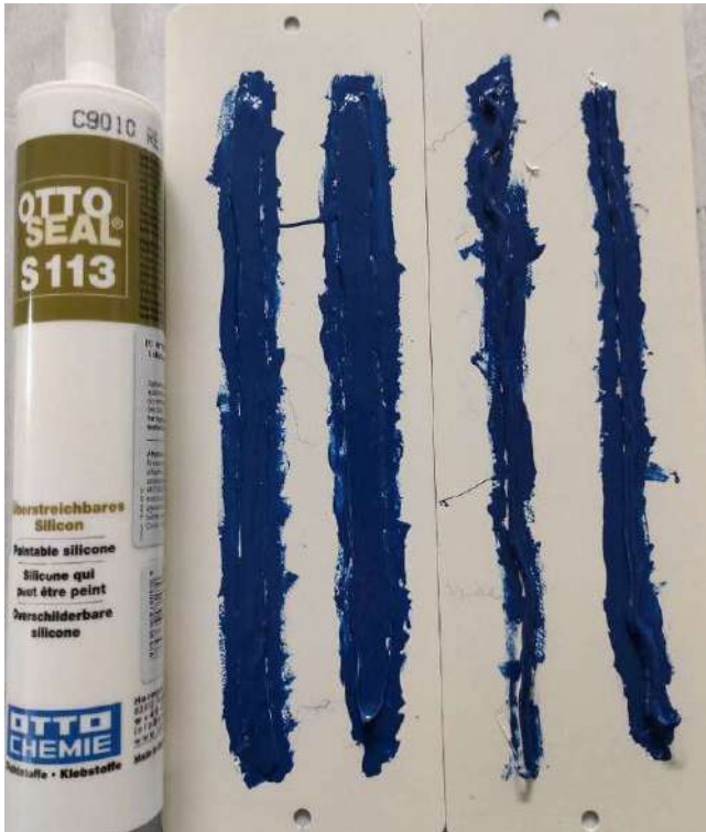
Figure 14 – 15: Results of the Touch-Up paint adhesion test on silicone.
