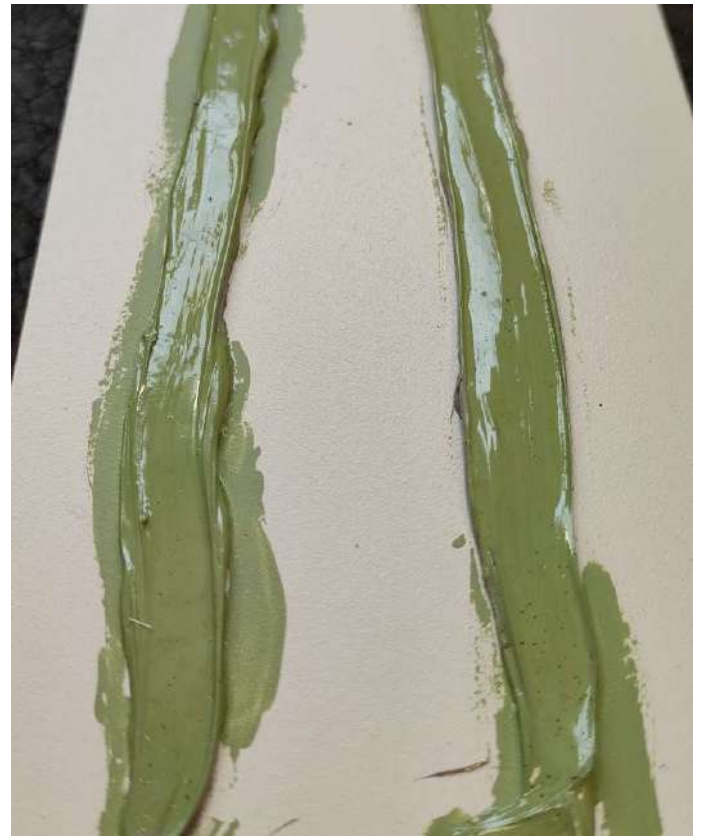
Figure 16 – 17: Results of the Touch-up paint adhesion test on silicone.
