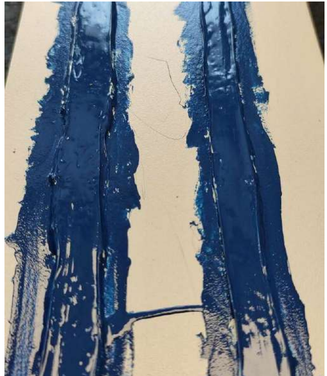
Figure 14 – 15: Results of the Touch-Up paint adhesion test on silicone.
