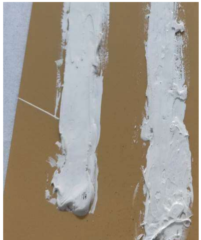
Figure 18 – 19: Results of the Touch-up paint adhesion test on silicone.
