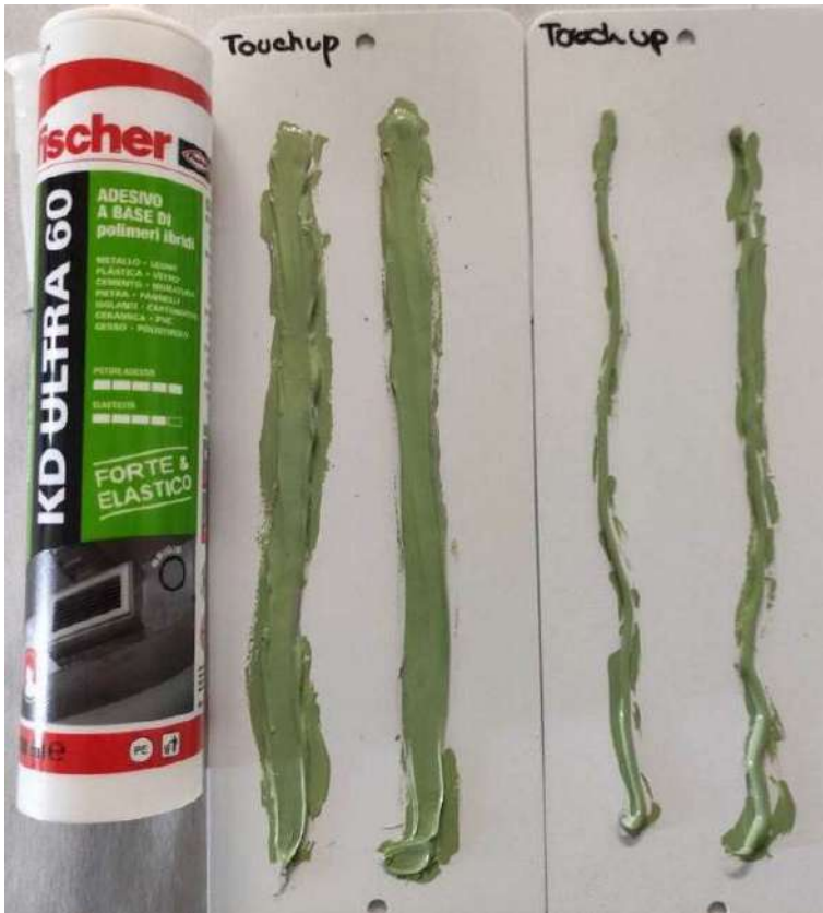
Figure 16 – 17: Results of the Touch-up paint adhesion test on silicone.
