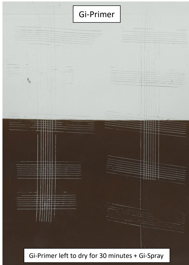
Picture 9: Adhesion test done on a sample panel, coated with high thickness of Gi-Primer.
