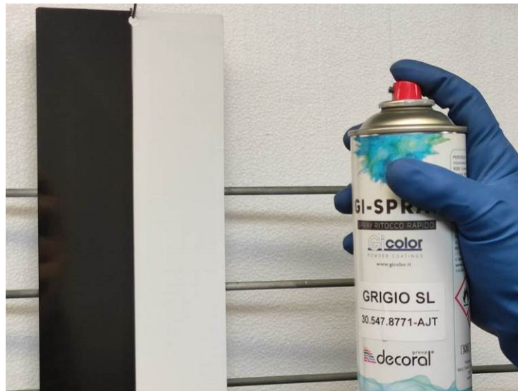
Picture 3: Sample panel before the application of Gi-SPRAY
