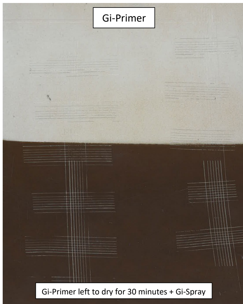
Picture 8: Adhesion test of Gi-Spray on a panel, coated with low thickness of Gi-Primer.
